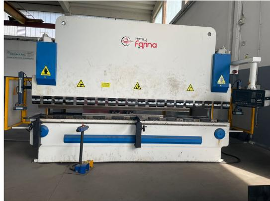
**PRESSA PIEGATRICE "FARINA" USATA, MOD. PSN 110/40, LUNGHEZZA DI PIEGA 4100mm, POTENZA 110TON, 4 ASSI, N.4 PUNTALI, INCAVO 500mm, CNC DELEM DA65, FOTOCELLULE DI SICUREZZA DSP NUOVA ELETTRONICA, BOMBATURA IDRAULICA, ANNO 2002, S.N. 691202/PA, CE**
