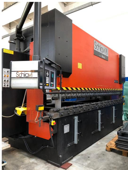
PRESSA PIEGATRICE IDRAULICA "SCHIIVI" USATA ,MOD. HFB 125/40 LUNGHEZZA UTILE 4100mm, POTENZA 125TON,INCAVO 410 CNC SIRIO TASK 84, 4 ASSI (Y1, Y2, X, R), ANNO 1997, CE, S.N. 970009-071-7240, PESO 10500KG
