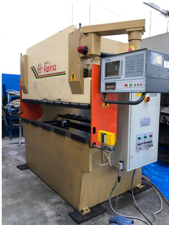
**PRESSA PIEGATRICE IDRAULICA SINCRONIZZATA "FARINA" USATA**, MOD. PFO/PS/N 40/20, LUNGHEZZA DI PIEGA 2100mm, POTENZA 40TON, 4 ASSI, N.6 PUNTALI, INCAVO 300mm, CNC ESA KLETRA 205, S.N. 4100395/S, ANNO 1995, CE
