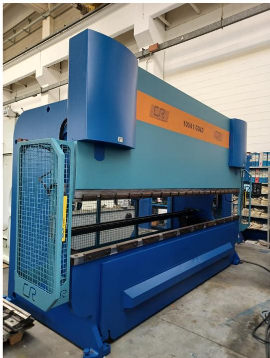
PRESSA PIEGATRICE IDRAULICA "CR" USATA, MOD. GOLD-100-41, LUNGHEZZA UTILE DI PIEGA 4100mm, POTENZA 100TON, CNC DELEM DA 65 VIDEOGRAFICO, FOTOCELLULE A BARRIERA, 4 ASSI, BOMBATURA IDRAULICA, INCAVO 510mm, ANNO 2002, S.N. P050602, CE
